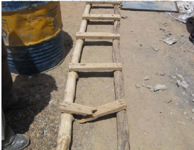
Bad hand tools Unsafe tools
